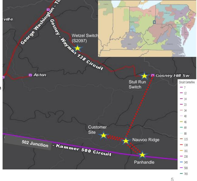
Construct a new 1.5 mile double-circuit 138kV line from Panhandle to Nauvoo Ridge. Utilize 1033 ACSR conductor for each circuit. Acquire new right-of-way. Estimated Cost: \$5.0 M (s2270.6)
