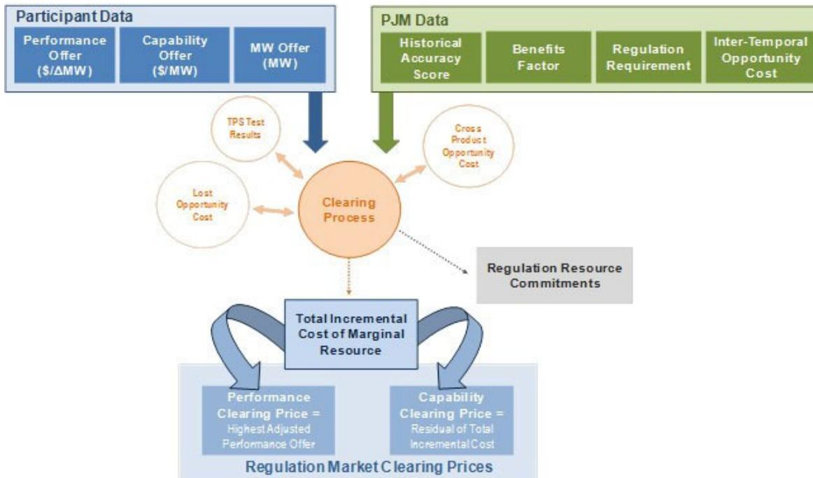
Each MCE, as described in Sections 2.5 and 2.7 of this Manual, ranks all available regulating resources in ascending merit order price, and simultaneously determines the least expensive set of resources necessary to provide Energy, Regulation and Synchronized Reserves for the operating hour taking into account any resources self-scheduled to provide any of these services. The Rank Price is determined as follows:
