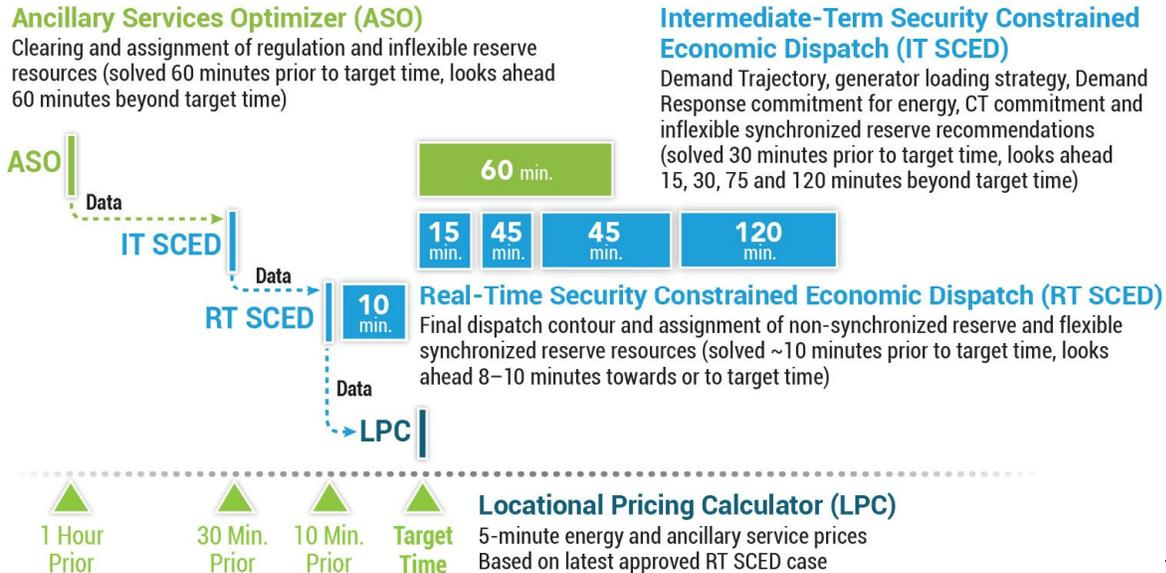
The applications jointly optimize the products for a defined target time to ensure that all system requirements are met using the least cost resource set therefore minimizing production cost.
