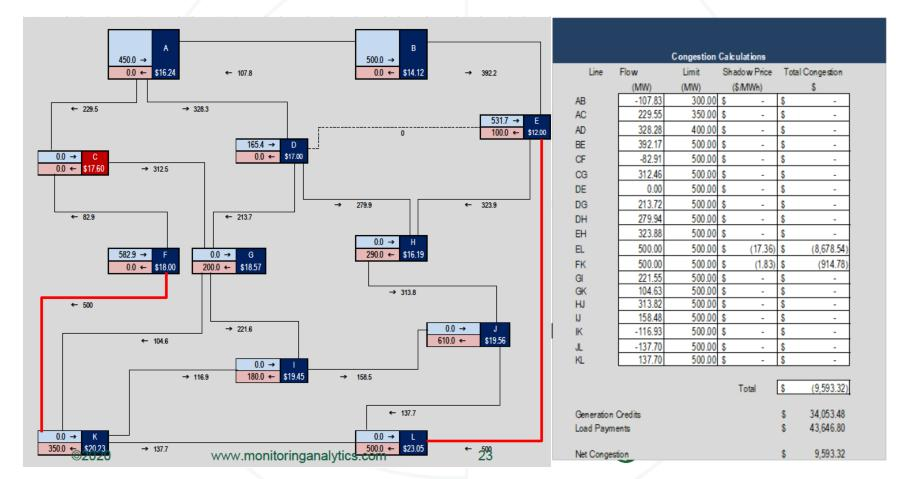
Bus E is closest to the source side of the constraint
