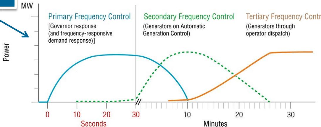
VG may displace conventional units & **reduce system inertia & primary frequency response**
