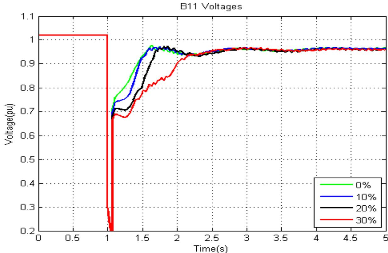
**As PV Increases → Voltage Recovery Increases**
